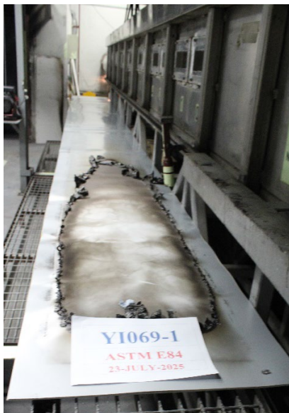
Photo 3: Specimen after the test. (As seen from the fire-end)
