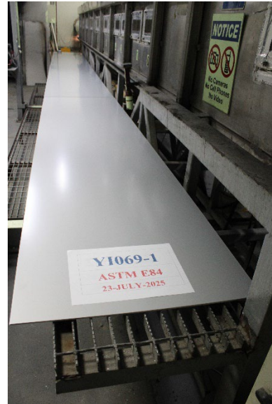
Photo 2: Specimen before the test. (Fire Side)
