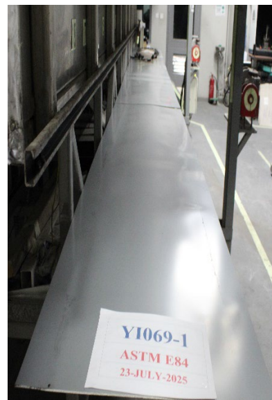
Photo 4: Specimen after the test. (As seen from the exhaust end)
