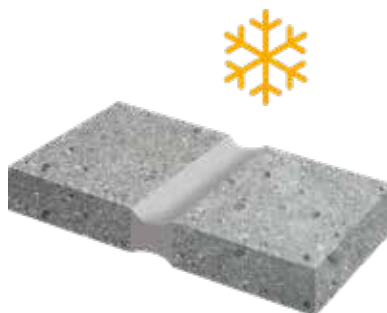
Contraction of building elements
